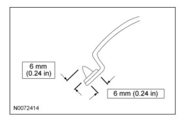
WARNING: Do not drive vehicle until the urethane adhesive seal has cured. Follow urethane adhesive manufacturer's curing directions. Inadequate or incorrect curing of the urethane adhesive seal will adversely affect glass retention. Failure to follow these instructions may result in serious injury to vehicle occupant(s).
